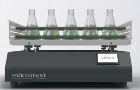
Orbital shaker is laboratory device that is used to shake liquids in closed vessels such as flasks, test tubes, bottles, culture plates, etc. This shaker is widely used in chemistry, biochemistry, molecular biology, microbiology and other scientific research laboratories.
