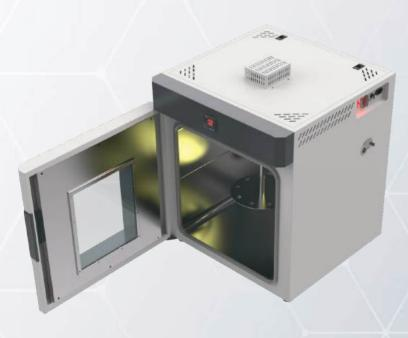
The Control System is digital PID controller. A built-in timer controls test times. Precision temperature control is easily programmed for test temperature, maximum temperature rating of up to 250 C. The oven is equipped with a dual safety thermostat to prevent accidental overheating. The plate rotates at 5-6 rpm.
