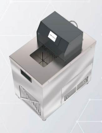
A refrigerated circulator is a device that maintains the temperature of a bath by circulating liquid through it. It consists of a bath, a refrigeration system, a heating system, and a pump to circulate the liquid. The bath is filled with a liquid, such as water and alcohol, which is circulated through the system. The refrigeration system cools the liquid, while the heating system heats it up, maintaining a specific temperature range.
