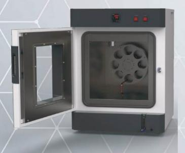
The Control System is digital PID controller. A built-in timer controls test times. Precision temperature control is easily programmed for test temperature, maximum temperature rating of up to 250°C. The rear inside wall is equipped with a vertical carriage, rotated by an electric motor at 15 1/min.
